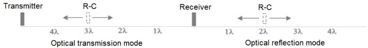
Fig. 4 Experimental layout for investigation of the damping efficiency of EMR by means of two-dimensional R-C
