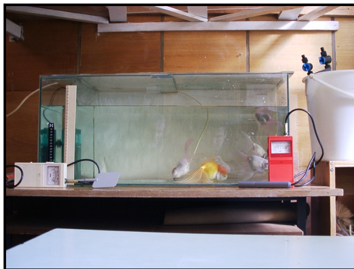
Fig. 8. Measuring EMF by magneto-metric instruments in aquarium area
