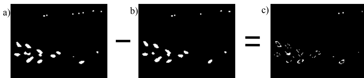
Fig. 5. Subtract two consecutive frames: a) и b) two consecutive frames after thresholding and filtering; c) difference frame.
